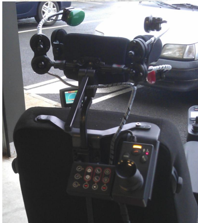
Power wheelchair with dual control and with a head rest control with 4 contacts
