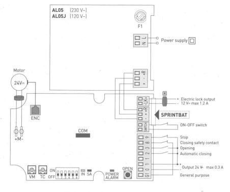
indicates where to install supplied ferrites as shown in figure
