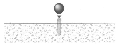
Fasten to the floor the floor doorstop as a mechanical stop in opening
