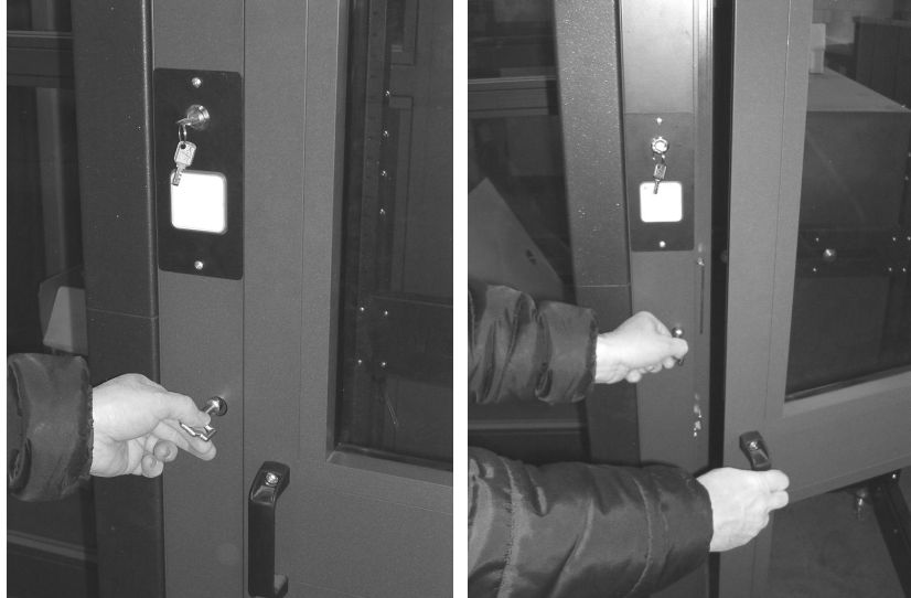
External unlocking door by emergency key
