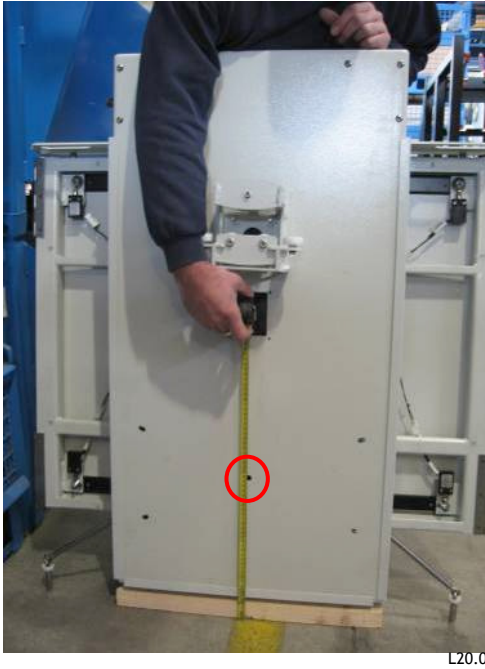
Measuring of the height of the central bore for the connection to the lower carriage
